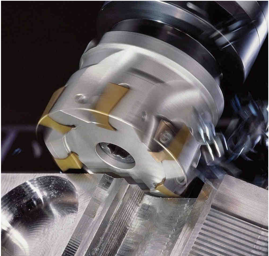
Machining of TVH® TV6082 aluminium alloy part
